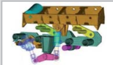
▲ Stinger rollers structural analysis
