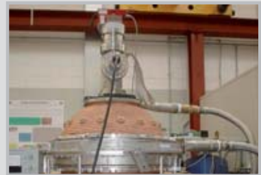
▲ Vacuum Test for 2 MW, 170 GHz Calorimetric Matched Loads (ITER)
