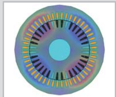
▲ Magnetic Flux line distribution inside an electric motor
