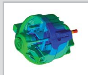
▲ Displacement contour map at the working frequency
